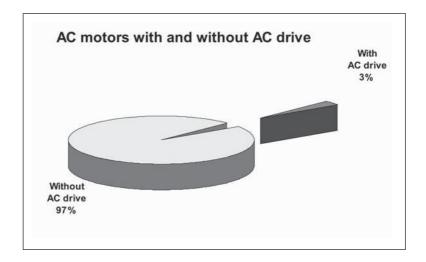
At the moment there are still plenty of motors sold without variable speed AC drives. This pie chart shows how many motors below 2.2 kW are sold with frequency converters, and how many without. Only 3 percent of motors in this power range are sold each year with a frequency converter; 97 percent are sold without an AC drive.
