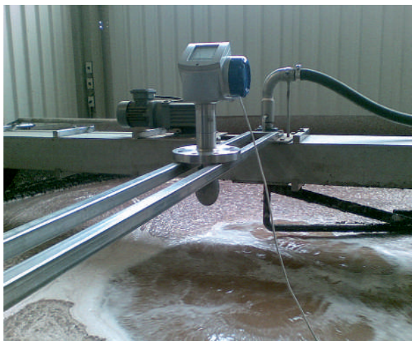
The OPTIWAVE 7300 measures the reflectivity of the product surface
