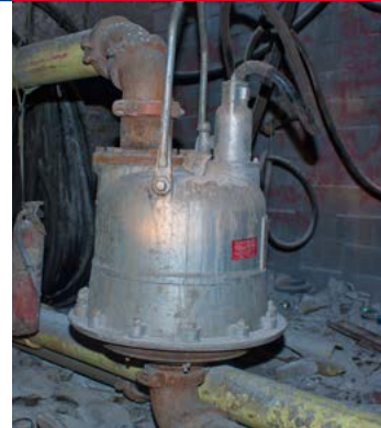
In-line staged submersible pump increases pumping distance.
