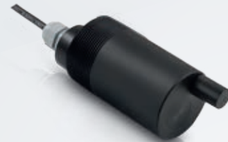
OPTISENS TUR 2000 90° scattered light sensor for turbidity measurements with NIR-LED for long-term stability and automatic cleaning
