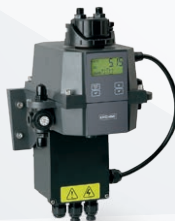
OPTISYS TUR 1050 Turbidity measuring system with cost efficient cuvette calibration and automatic ultrasonic cleaning system
