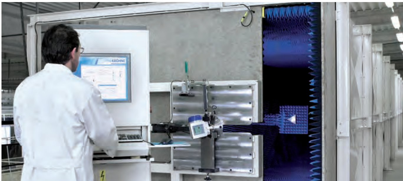
Stretch for calibration of FMCW level transmitters
