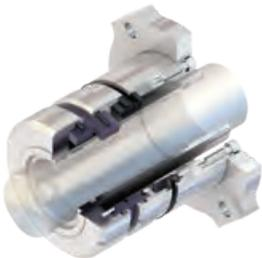
The RIS rubber-energized, component slurry seal features a unique non-clogging design that does not utilize springs or bellows. Handles solids to 50% by weight.
