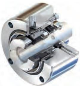
HSH balanced, flexible stator cartridge seals are built for extended reliability in high-pressure, high-speed and highly viscous services such as crude oil pipeline pumps. Fully compliant with API 682 Type A, Arrangements 1, 2 and 3.
