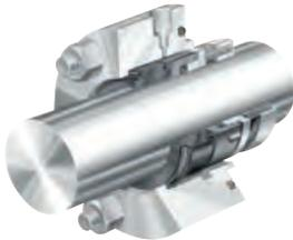
This single, unbalanced, multi-spring component seal is usable as an inside or outside mounted seal. Suitable for abrasive, corrosive and viscous fluids in chemical services.
