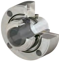
This medium- to high-pressure seal features a high balance face that meets the lowest light hydrocarbon emissions level: less than 500 ppm. Designed to suppress flashing and minimize heat generation.
