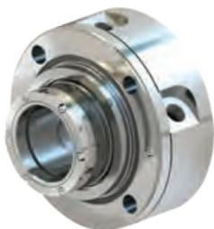
GSDH seals are dry-running metal bellows containment seals for high-temperature hydrocarbons, heat transfer fluids and other fluids pumped beyond the temperature limits of elastomers.
