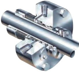
These robust balanced metal bellows seals are designed for high-temperature hydrocarbons, heat transfer fluids and other severe services. Meet all API 682 Type C requirements in Arrangements 1, 2 and 3.
