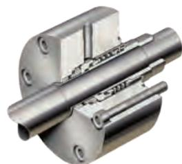
D Series single spring, balanced pusher seals have a high-circulation integral pumping ring to ensure proper cooling. Ideal for high-temperature boiler feed water and hot hydrocarbon services.
