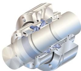
This dual pressurized, high-temperature metal bellows gas seal is engineered for the hottest process pumps found in refinery and hydrocarbon services. Qualification tested per API 682 Type C, Arrangement 3 requirements.
