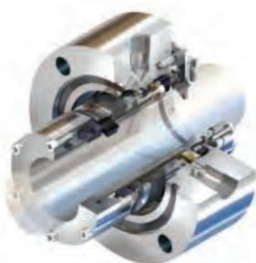
Built for temperatures beyond the limits of elastomers, the BXRH balanced stationary metal bellows seal offers reliable sealing at high speeds. Meets all API 682 Type C requirements in Arrangements 1, 2 and 3.
