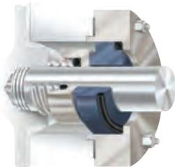
The CRO is an economical, single-coil spring, friction drive component seal for use in pumps with packing box seal chambers. Available in single or dual arrangements.
