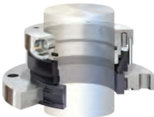
The VRA is an outside-mounted, dry-running single pusher seal designed to operate on top-entry agitators and mixers. Self-lubricating carbon or filled PTFE seal faces run completely dry without cooling.
