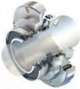
SLC seals are heavy-duty, single pusher cartridge seals built for the harshest slurry pump services found in mining, mineral and ore processing, and flue gas desulfurization. Suitable for solids to 60% by weight.
