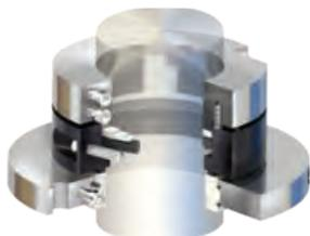
The MSS is for tough mixer and vessel applications where stuffing box face bore and OD run-out are extreme. Typically used on older equipment or where compression packing had been used.
