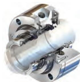
BXHHS and BXHHSB balanced rotating metal bellows seals are designed for refinery and petrochemical services at high- and low-temperature extremes. Meets API 682 Type C requirements in Arrangements 1, 2 and 3.
