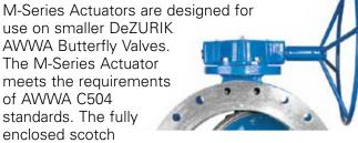
yoke mechanism allows the M-Series Actuator to provide a torque curve that matches the torque requirements of the valve. The thread system of the traveling nut is self-locking, maintaining disc position under varying flow conditions.
