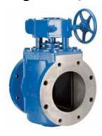
Eccentric PEF Plug valves comply with AWWA C517 and are capable of handling clean and dirty liquids and gases, sludge and slurries. Port is 100% of standard pipe area, including straight through body design with flushing port to maximize flow capacity and reduce head loss. Rectangular port design provides wide tolerance seating geometry
