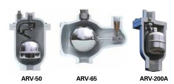
Air Release Valves function to release air pockets that collect at each high point of a pressured pipeline, and are essential for pipeline efficiency and water hammer protection. Air Release Valves are available in a wide variety of orifice sizes and materials of construction to meet a wide range of applications.
