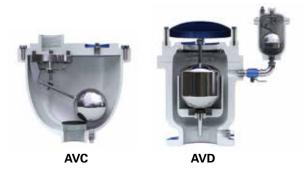
Release Valves and Air/Vacuum Valves. Combination Air Valves are installed on all high points of a system where it has been determined dual function Air Release and Air/Vacuum Valves are needed to release air and also protect the pipeline from vacuum. Combination Air Valves are available in two body styles: single body combination or dual body combination. The single body combination is used where compactness is preferred.
