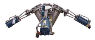
Mixing and Diverting Knife Gate Valves are available with either an integral body or a replaceable body. Valves with the replaceable body design are bolted to a Y-pattern pipe, allowing easy replacement of a single valve rather than the entire assembly.
