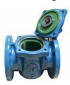
In applications where mineral build-up can be an issue, Glass Lined PEC or PEF Eccentric Plug Valves provide a smooth, non-stick glasslined interior that can inhibit crystalline formation inside the valve. Glass Lined valves are commonly used in wastewater treatment plants where Struvite
