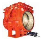
metal or resilient. The valve comes equipped with a bolted cover which can be removed while the valve is in the line. The connection between the disc and disc arm allows disc to move for precise alignment with the seating surface. The valve is available with external counterweight and bottom mounted buffer.
