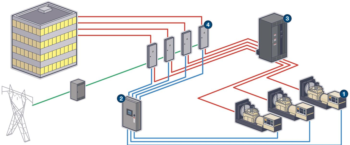
The KOHLER® Decision-Maker® Paralleling System (DPS) offers a truly integrated approach to generator paralleling. Each system includes generators, Decision-Maker 6000 controllers, a master control panel, power distribution switchboards with breakers and KOHLER automatic transfer switches.
