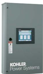
Responsible for generator and load management, the master control panel handles load add/load shed; number of gensets online; and also monitors electrical and mechanical loads along with event logging and alarms.
